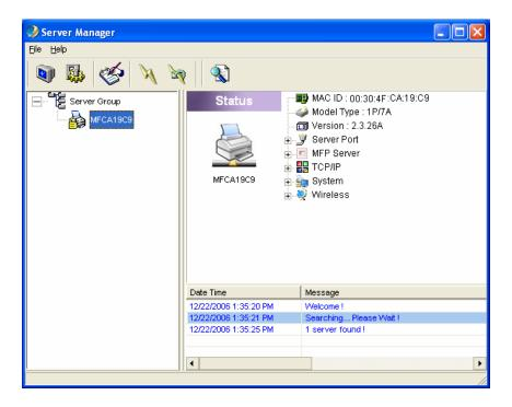
Click "Status" icon on the tool bar, the status of the currently selected MFP Server will be showed on the right side of the window. The information of the MFP Server displayed are including MAC ID, Model Type, Firmware Version, status of each server port, IP address, subnet mask, default gateway and supported printing protocols...etc.
